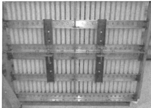
Figure 4-28. Both sides of the cassette should have two jacks attached.
